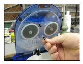
1. Find a small container or use a piece of paper towel to catch water and compound from the nozzles during the priming process.
