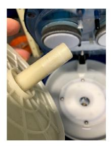
Remove platen by lifting it straight up and out
